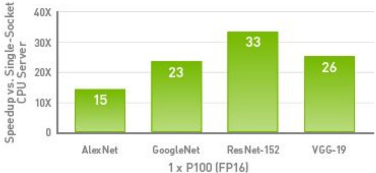
CPU Server: Single Xeon E5-2690 v4 @ 2.6GHz | GPU Servers: Single Xeon E5-2690 v4@2.6GHz with 1xP100 (PCIe) | Ubuntu 14.04.5 | TensorRT 2.0 | CUDA 8.0.42 | cuDNN 6.0.5 | NCCL 1.6.1 | Batch size 128 | Precision FP32 (CPU) | FP16 (P100 GPU).
